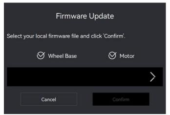
Click the ">" button on the right side of the pop-up window to select the firmware you have downloaded for the corresponding product; in the pop-up window, select the corresponding firmware type ("Wheel Base" or "Motor"), then click "Confirm" to update the firmware.
